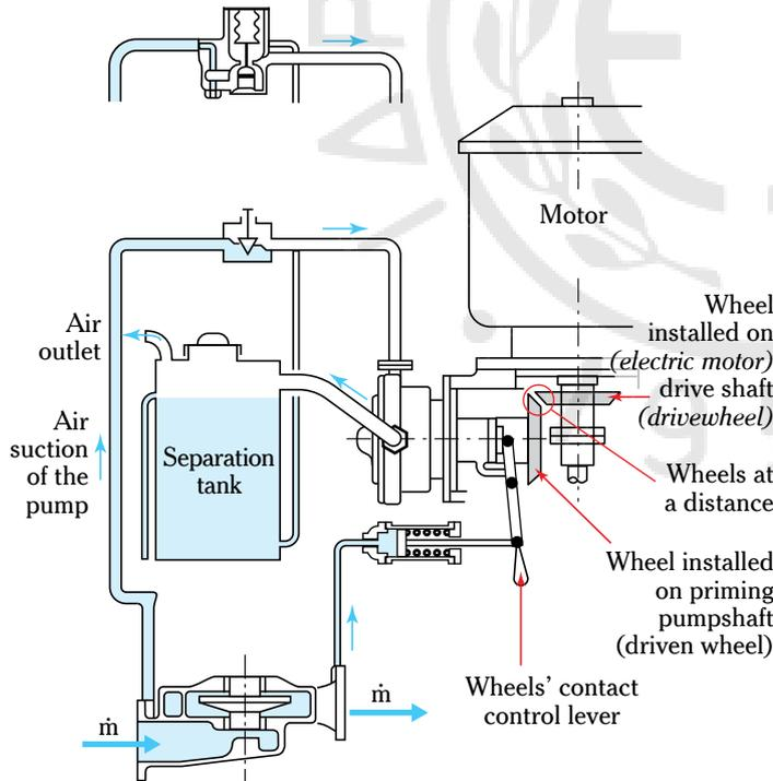
Pump with water, after the removal of air
