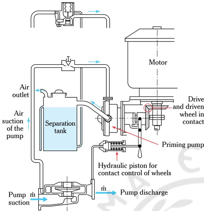
Pump during starting, with air inside
