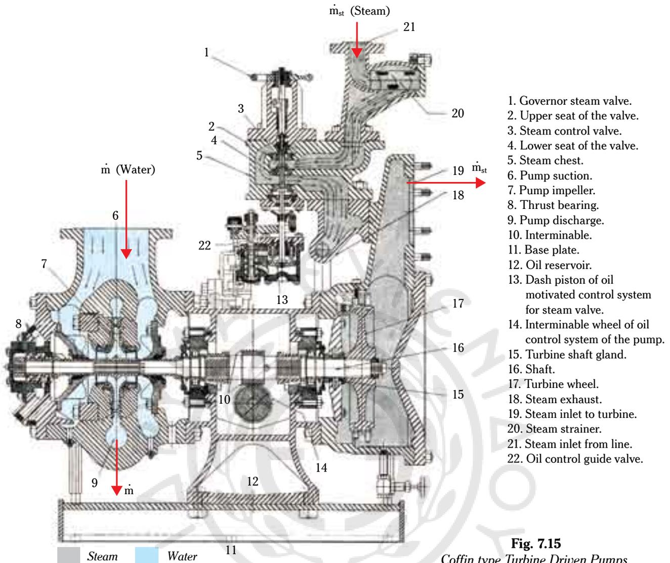
ball bearing type, which is placed in the outer casing. This provides automatic adjustment of the axial position of all the moving parts, without having to use plug-ins or other regulatory instruments.
