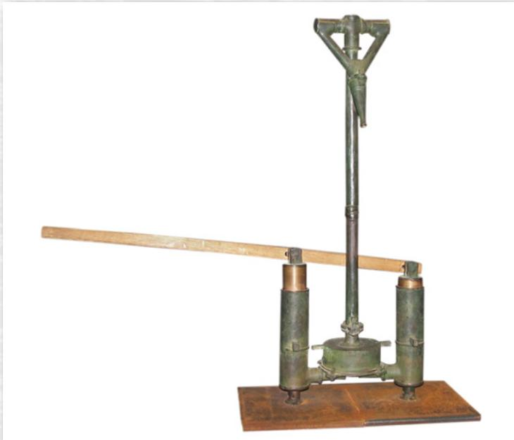
*Working model of a Ctesibius piston pump.
