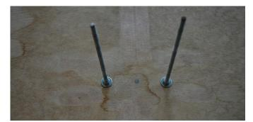
Figure 12. Grip the threaded rods using nuts and washers
