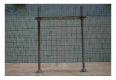
Figure 14. Nuts and mending plate attached to the threaded rods
