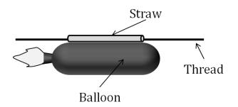
Figure 5. Balloon taped to a straw which is threaded onto a string
