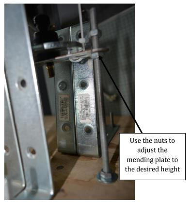
Figure 22. How the nuts under the mending plate can be used in order to attach it to the desired height, so that the nails will pass smoothly but firmly above the wide neck lip
