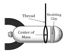
Figure 36. How to find the center of gravity of a water rocket
