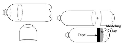
Figure 27. Cut the top part of the second bottle and remove the nozzle as shown in the figure.
