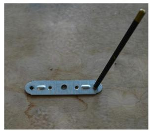
Figure 9. Mending plate on wooden base. Holes are marked using a pencil.
