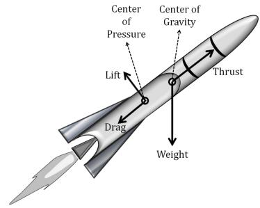
Figure 37. Forces acting on a rocket during flight.
