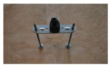
Figure 15. Mending plate and rubber stopper with valve attached to the threaded rods
