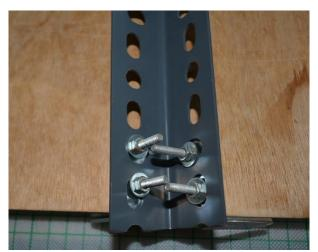
Figure 23. Small steel brackets attached to a Dexion angle
