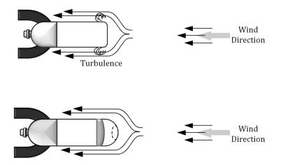
Figure 35. Wind behavior flowing around a bottle without and with a nose cone. Watch the turbulence which is created in the case of the bottle which doesn't have a nose cone. Turbulence influences rocket's aerodynamic behavior.
