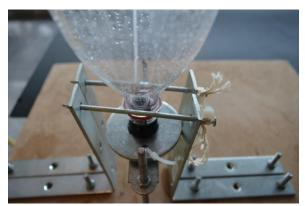
Figure 21. Steel nails pass smoothly but firmly above the wide neck lip
