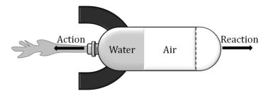
Figure 34. Newton's third law in the case of a water rocket.
