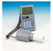
and built by engineers who work in biomedicine. <u>One such instrument, used for measuring</u> <u>lung volume, is the **spirometer**</u>.
