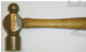
Ball-peen (peen) hammer a hammer with one end of the head flat and the other end rounded, used for forming soft metal
